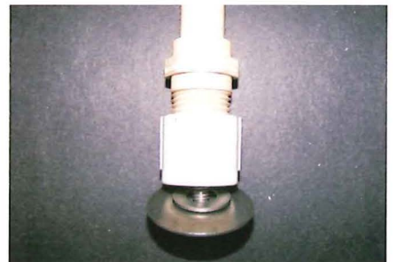
The large washer and small washer ride against the carriage bolt head.
