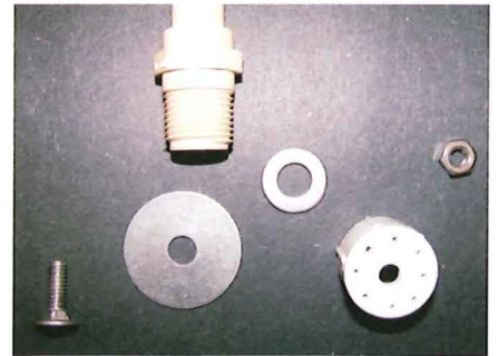
A carriage bolt (far left) holds the assembly together.
